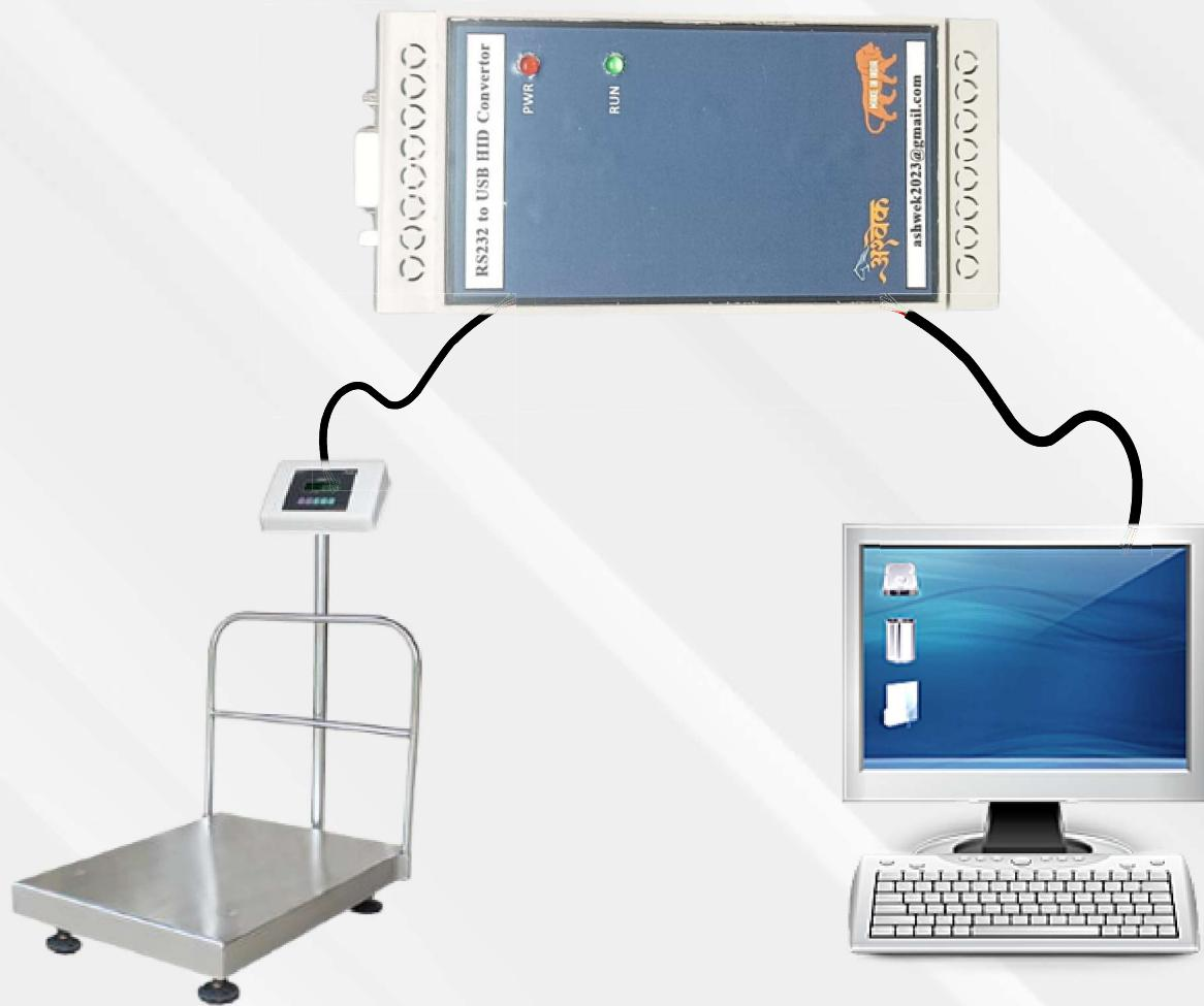
**WEIGHT DATA IS DIRECTLY TRANSFERRED TO THE CURSOR IN REAL-TIME,
